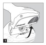
2 Open the film door by pushing the blue film door button.
